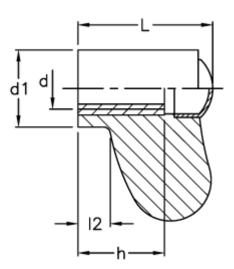
$$\begin{array}{lll} b & = 8 \\ d1 & = 16 \\ d \ 6H = M8 \\ h & = 18 \\ L & = 28 \\ l2 & = 6.5 \end{array}$$
